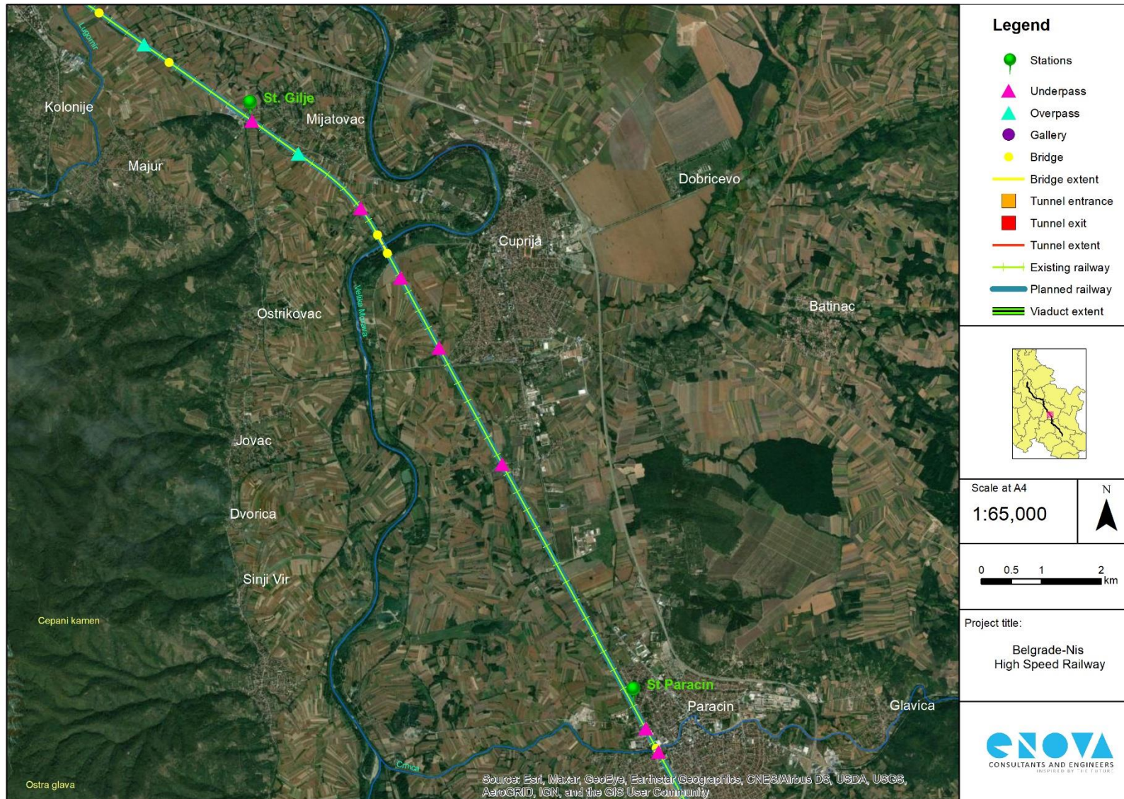
Figure 8: Existing and planned railway with ancillary structures (Gilje-Paracin subsection)
